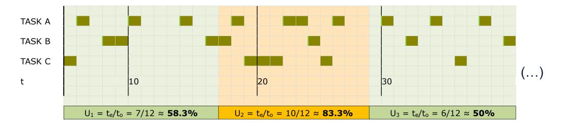
Which of the CPU loads is 'the' CPU load? Max? Average?
